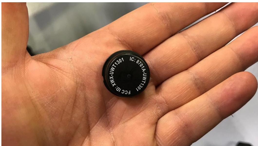
This is quite different from GPS-based solutions. Zebra says their solution is more accurate, measured within 15 centimetres, whereas GPS is within metres. Also, the Zebra solution is designed for indoor use whereas GPS is less effective as it requires line of sight to the satellite network.
